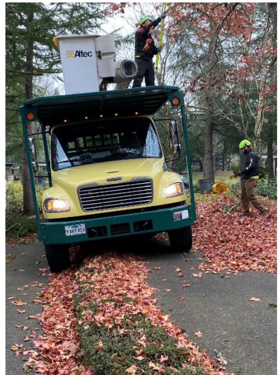
Bartlett trims the Fire Lane at OPV. LO requires that fire lanes be cleared up to 16 feet so that fire trucks can easily pass.
